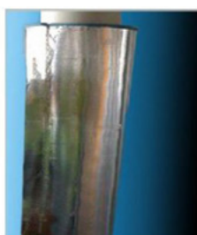
Tape along the longitudinal overlapped length
